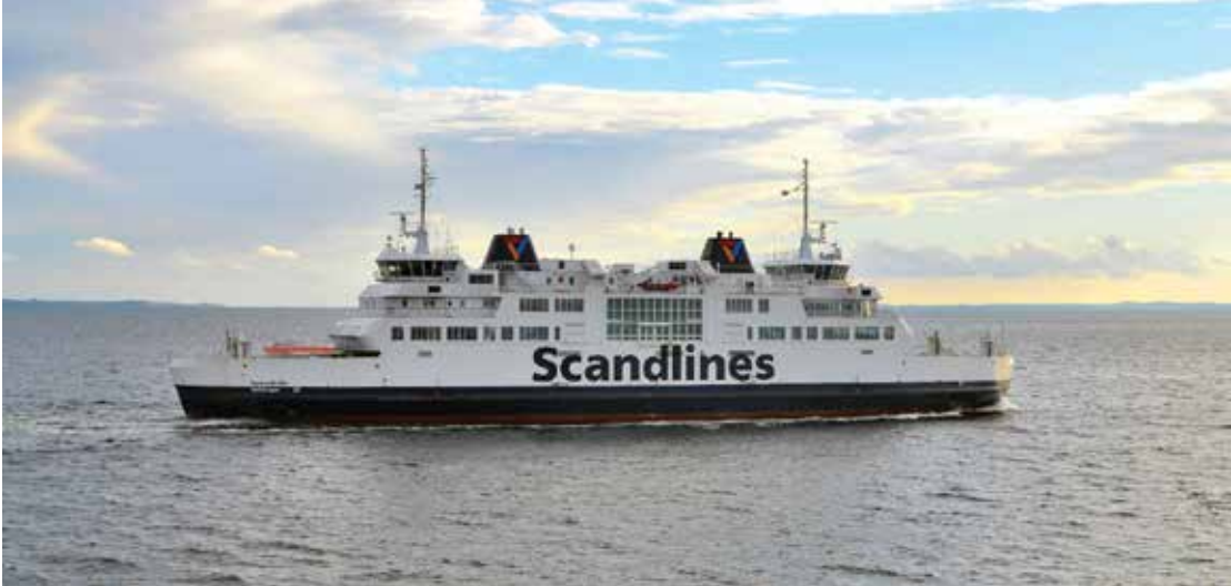
Figure 2: PBES batteries are found in the world's largest fully electric vessel, Tycho Brahe. The 12,000 ton, 266 m electric ferry has a 4.2 MWh battery that is capable of completing the 45 minute crossing between Denmark and Sweden three days on one charge.
