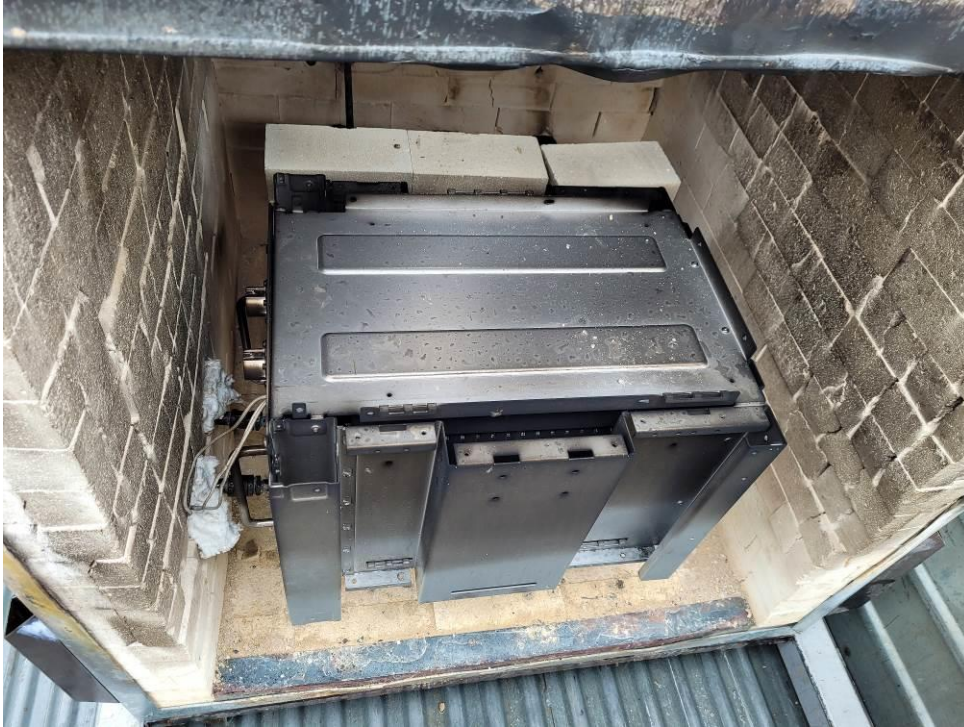
Picture 8 – Unit BBU – Unit After Exposure at 215°C
