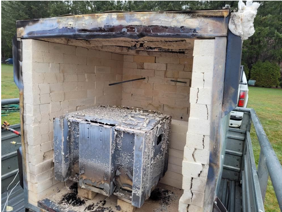
Picture 9 – Unit BBU – Unit After Exposure at 950°C
