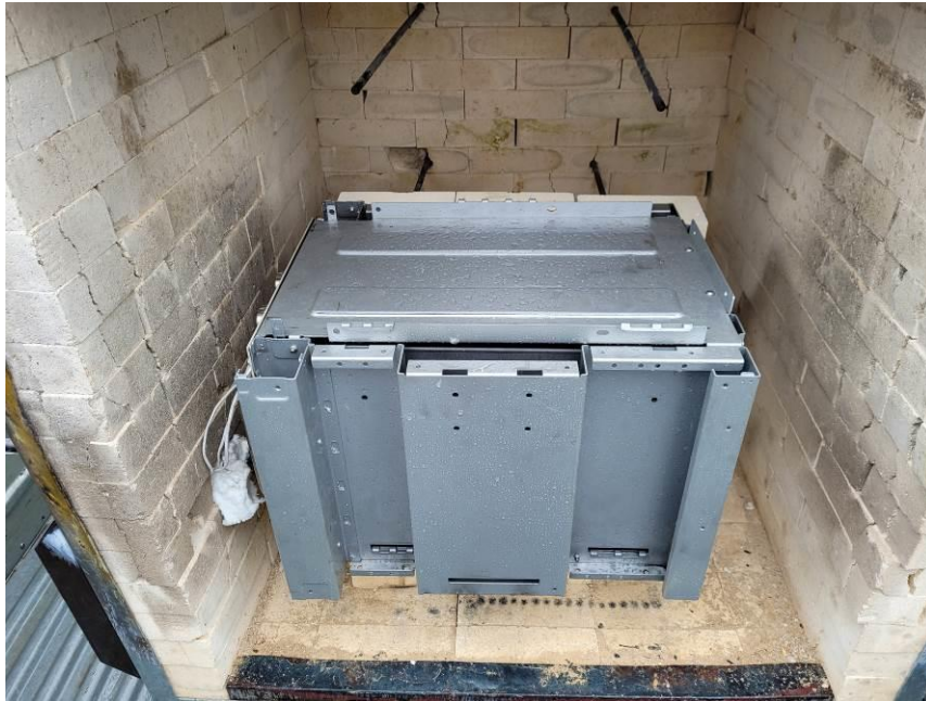
Picture 7 – Unit BBU – Unit Installed in the Chamber
